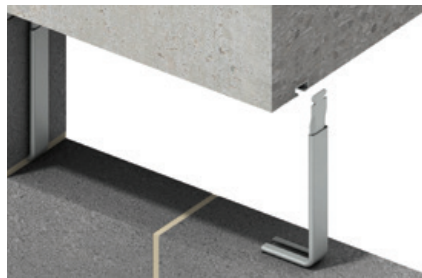
Ancon IHR - C Restraining Top of Inner Block Wall to 38/17 Channel Cast into Concrete
