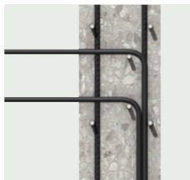
Traditional slab-to-wall construction method. Projecting reinforcing bars and congestion in the wall.
