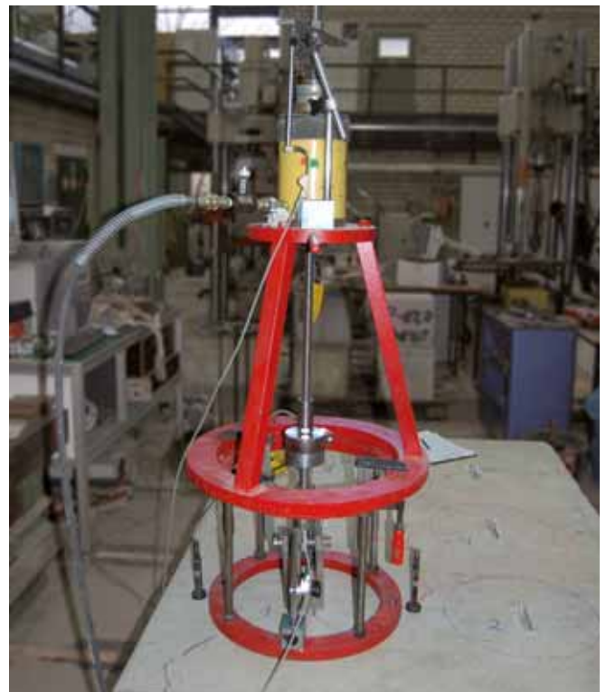
Test setup; pull-out test
