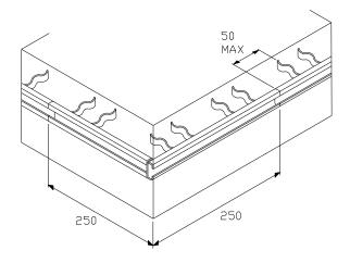
**Welded Corner Fabrication**
