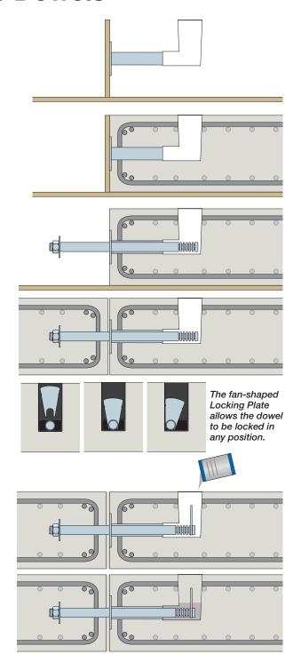
**Notes:** Where deep concrete pours are proposed, the installation will require further consideration. More robust fixing of the sleeve and dowel components will be necessary, to avoid displacement during casting of the concrete. Ensure joint has been filled before pouring resin.
